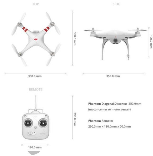
The Phantom uses the DJI NAZA-M flight control system, which provides auto level stability, altitude hold via onboard barometer and position hold via GPS. The GPS also is used in providing failsafe return to home safety feature. The system does NOT provide for waypoint navigation.
