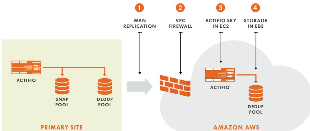
FIGURE 3 Low RTO Disaster Recoveries in AWS
