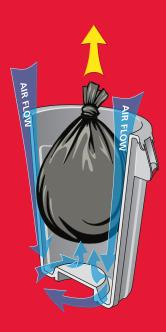
Patent-pending venting channels dramatically reduce the force required to remove a filled can liner—over 50% compared to traditional containers.
