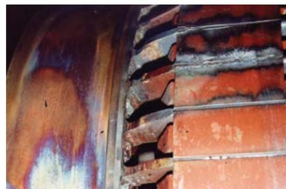
Rotor core damage due to broken bars
