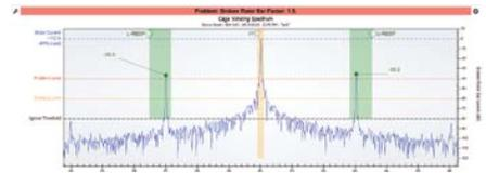
Broken rotor bar spectrum analysis
