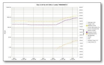
• Alarms triggered by exceeding rate of change limits allow for early detection of incipient faults.
