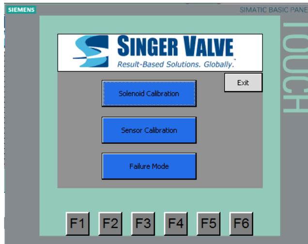
**\*\*\*WARNING: When making any changes to any calibration menus ensure that all process controls and manual control of the valve are off!!**
