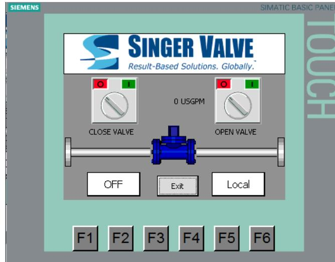
Toggling the LOCAL/REMOTE switch to the REMOTE position will give manual control to a remote system input. This will allow a remote SCADA input to have access to toggling the ON/OFF switch and the Open Valve and Close Valve toggles switches. Switching to REMOTE position will also disable the local user from being able to toggle the ON/OFF switch. To regain local control the LOCAL/REMOTE toggle needs to be put back to LOCAL
