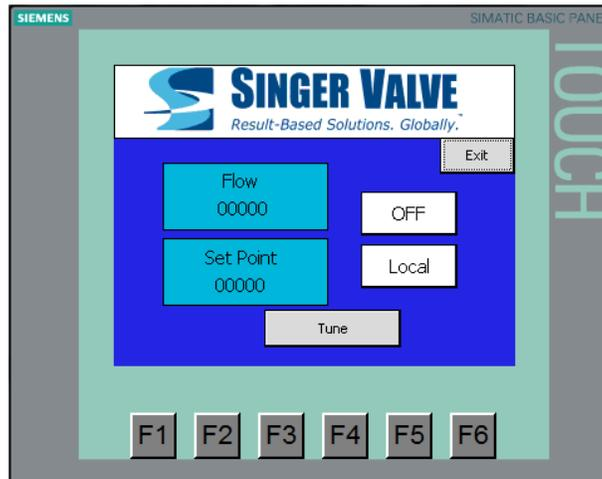
Toggling the LOCAL/REMOTE switch to the REMOTE position will allow the system to receive a remote set point. This will allow a remote SCADA input to have control over the valve process control. Switching to REMOTE position will also disable the local user from being able to toggle the ON/OFF switch. To regain local control, the LOCAL/REMOTE toggle needs to be put back to LOCAL
