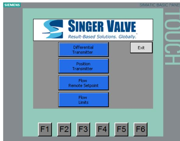
To calibrate a specific analog input signal touch the button matching that specific input. This will bring up the Calibration Window with the real time Analog Signal being received.
