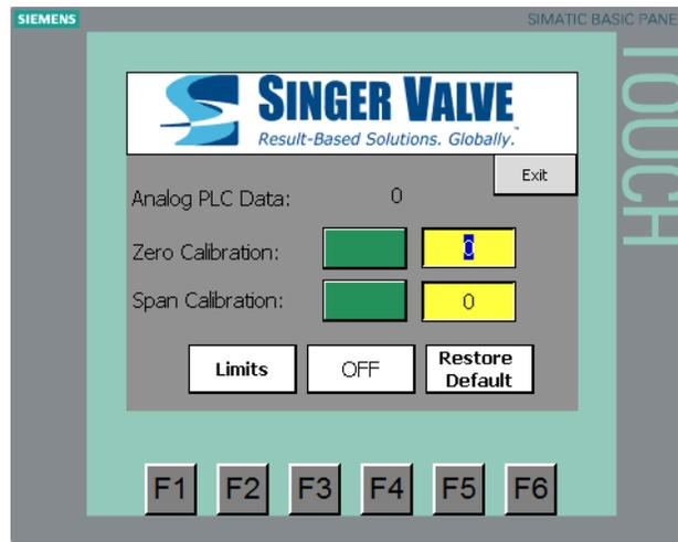
The PLC controller has an analog input that receives a 4-20mA signal from the Process Variables or Remote Control Set Points. The real time signal being received by the PLC is displayed in the Analog PLC Data field. This value should range from 5400 to 27600.
