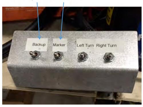
4.9.3 Keep marker lights on and flip switch on for left turn signal. When left turn is switched on, check to see that the left turn signal light gets a brighter illumination and light always remains on while running.
