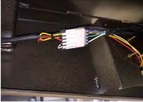
4.5.3 Take main harness line from tail light to rear side narjer and zip tie main harness to side marker wires.
