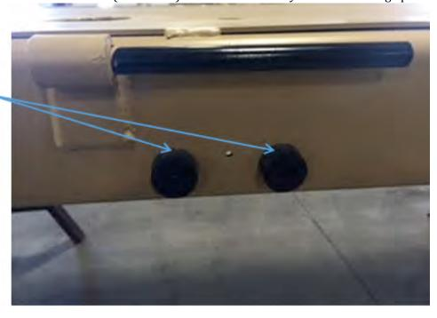
4.1.6 Attach two bumpers (79200009) on each end at rear of body underneath hinge pins.
