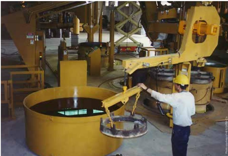
Dip tanks are used frequently in the pipe manufacturing industry as an efficient means of coating parts with form release agent.
