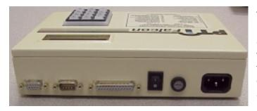
This is the rear view of the PTI Falcon Base Unit. The left most connector (RS485) is a 9-pin female connector and connects to the remote keypads and other remote devices. If door alarms are in use, the alarm relay contacts are also present
