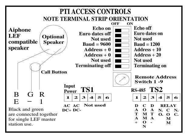
It is necessary to wire the following items to the remote keypad for proper operation:
