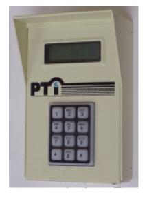
panel behind it for nighttime viewing. This light comes on when the "\*" key is pressed on the keypad to begin a transaction. The housing for all PTI keypads and card readers are all aluminum to resist rusting. To use the Remote Keypad to access the property simply press the star key (\*) then your access code and then the pound key (#).
