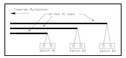
Method 3 is wired the same way a conventional alarm panel is by using 2 separate conductors for each and every door. A 22awg 2 Conductor cable is run to each door and terminated at each door switch. The opposite end in the mux is then punched down accordingly. Due to the limited number of grounds terminals available on the multiplexer it will be necessary to group some of them together then punch down a single wire.
