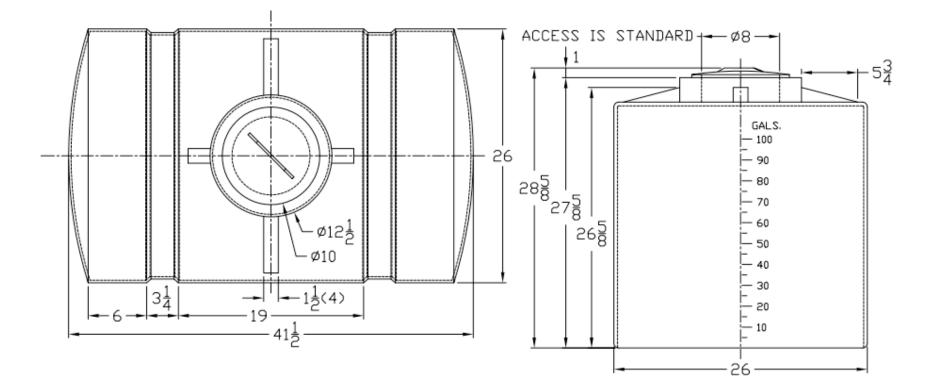
ALL DIMENSIONS SHOWN ARE OUTSIDE PART DIMENSIONS IN INCHES, AND VARY BY THE STANDARD ROTATIONAL MOLDING TOLERANCE OF  $\pm 2\%$ .
