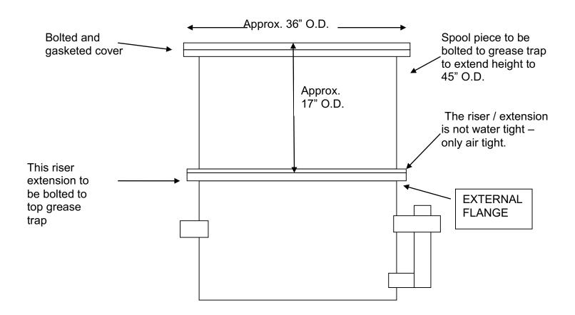
THIS IS AN EXAMPLE OF A RISER- THE ONE SHOW AS AN EXTERNAL FLANGE - (ON THE OUTSIDE) TO GIVE YOU AN EXAMPLE OF BOTH FLANGES.
