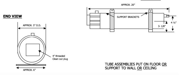
**NOTE**: Smaller Limestone Chips (Approx. ¼" Diameter) to be installed by Contractor. These special limestone chips (model #SLS-50) available from T&C. (One bag can fill 3 cartridges).
