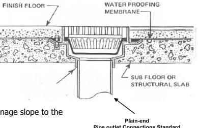
Pipe outlet Connections Standard (MPT outlet connections optional)
