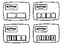
Set switches 1 through 9 at any security code, press and hold desired channel. Now press learn, The green LED will llash indicating the channel is stored. One flash is for channel one, two for channel two, three for channel three, and four for channel four. The transmitter has now stored the code in the corresponding channel until the learn switch is pressed again.
