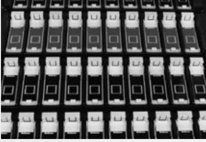
40 Independent Thermal-Cyclable Modules
