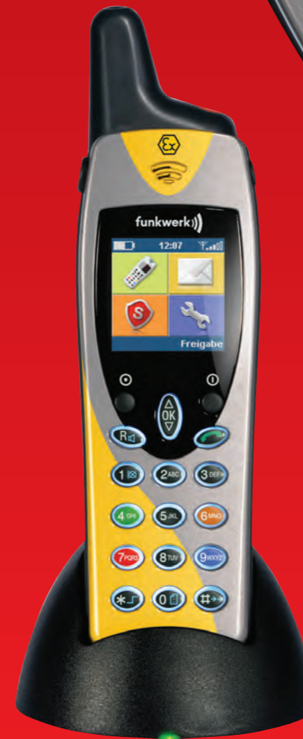
Clockwise from top left: Process monitoring straight to your handset; lone worker protection such as automatic check-calls, tilt switch and pull-cord; text messaging to both on- and off-site contacts; a normal cordless phone that sits on your desk.
