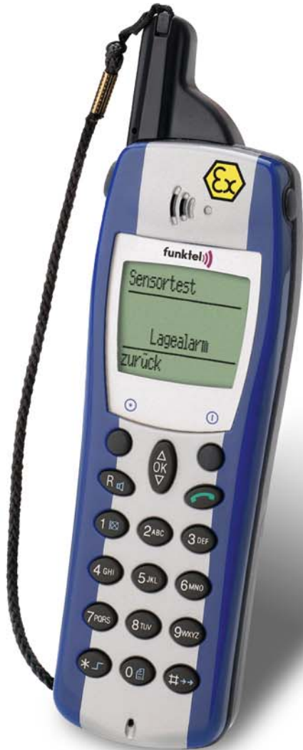
DSS personal emergency signalling unit funkwerk FC1 S Ex—with BG certification
