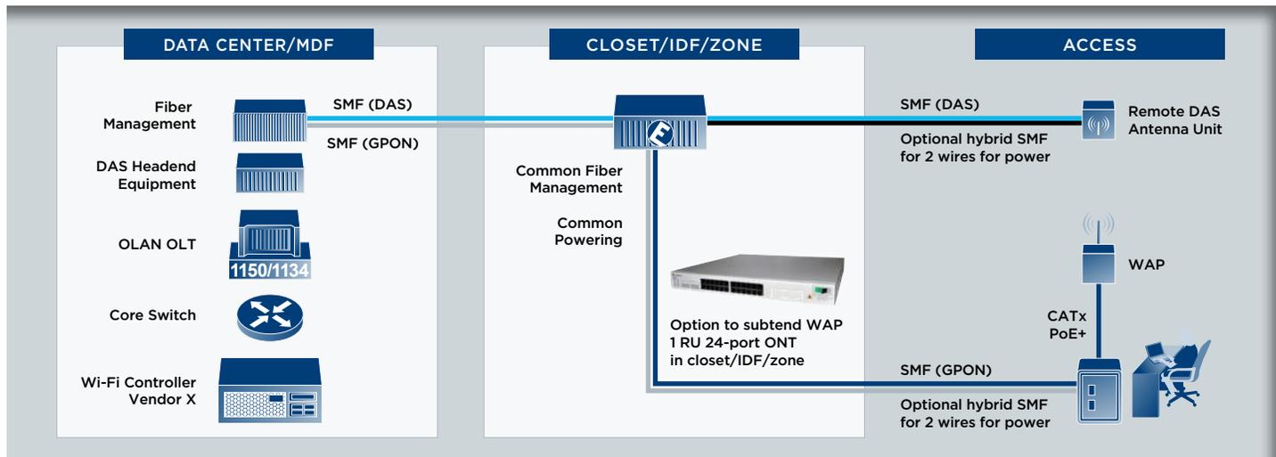
Figure 4: Fiber-based DAS solutions and Optical LAN architecture
