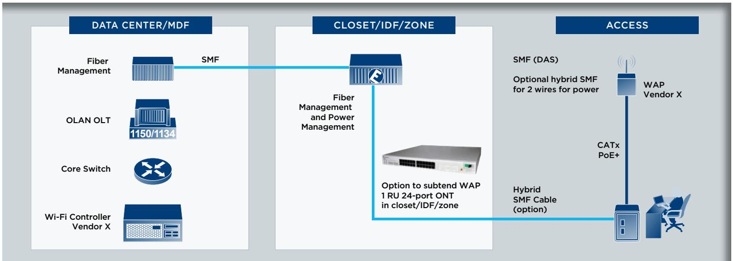
Figure 6: Fiber-based Wi-Fi solutions and Optical LAN architecture
