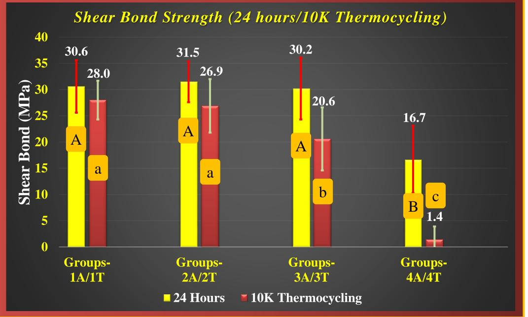
Crystallized Mounted Sectioned Polished Eighty specimens of lithium-disilicate (IPS e.max CAD) were sectioned, crystalized and mounted. Specimens were polished through 400 grit SiC paper. Specimens (n=10) were distributed in eight groups outlined in the table below [Group 1A-4A (24h) and Group 1T-4T (Thermocycled)].
