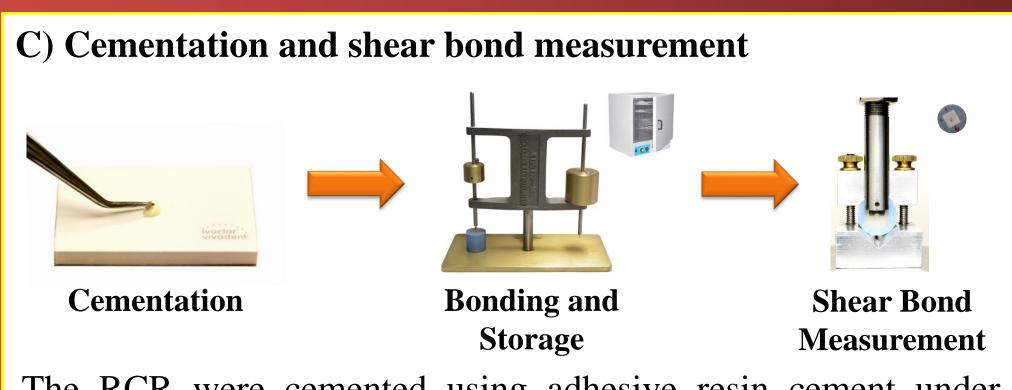
The RCR were cemented using adhesive resin cement under constant load (113.4 grams). Specimens were light-cured per manufacturer's instruction followed by storing for 24 hours at 37°C/100% humidity before shear-bond testing using universal testing device (Instron / crosshead speed-1.0 mm/min).
