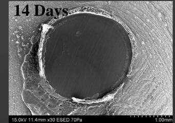
100% Adhesive failure between cement and ceramic surface
