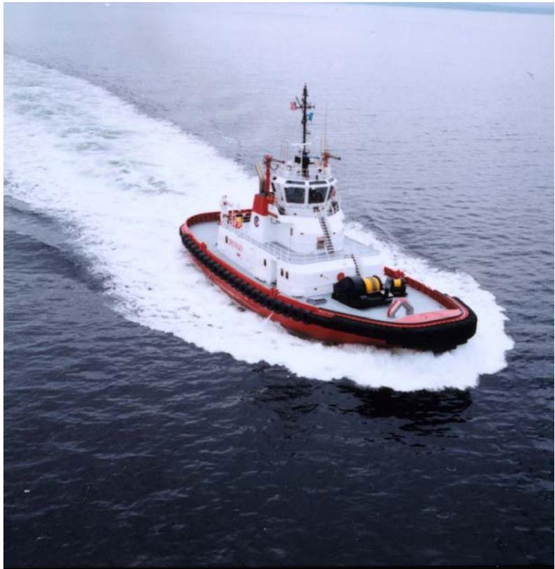
Data was being collected in hopes of determining the root cause of excessive hull vibration. To do this, several testing and analytical techniques were utilized. The DOE (design of experiments) encompassed operating factors of ballast level, speed, and structural points. In all cases, structural point data was collected simultaneously from a matrix of conditions decided upon before each sea trial.
