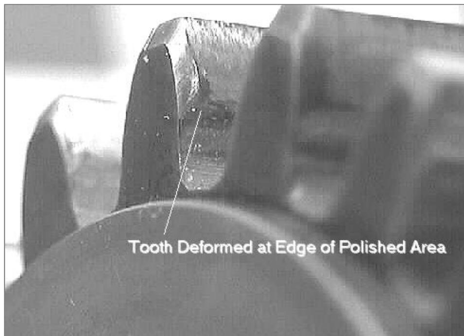
The figure above is a close-up of the edge of a damaged tooth. Note the upset metal at the end of the contact area.
