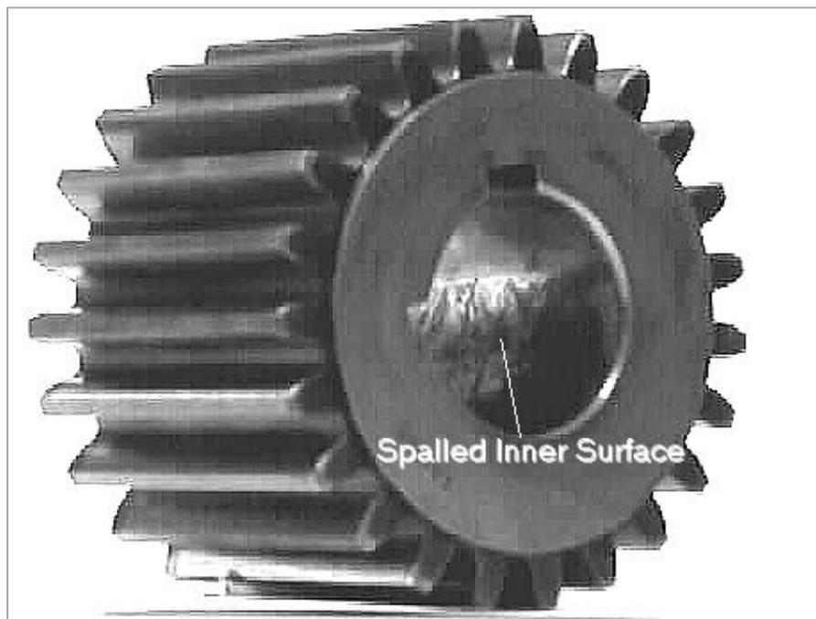
The figure above shows the spalling in the pinion bore caused by the gear turning back and forth on the shaft.
