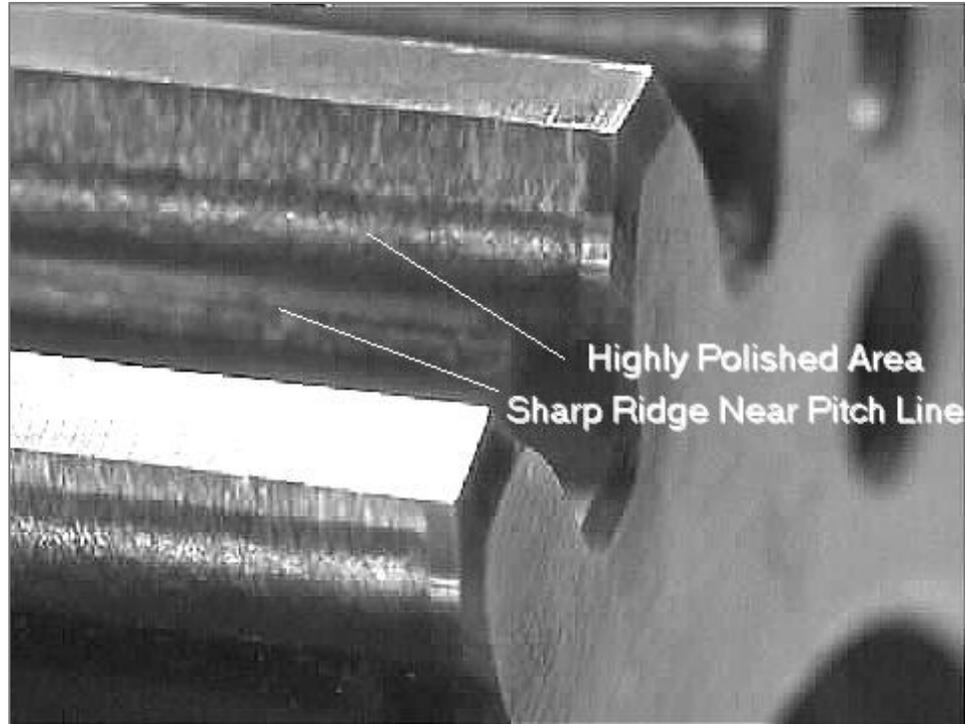
The figure above shows the abrading wear on the sides of the gear teeth.
