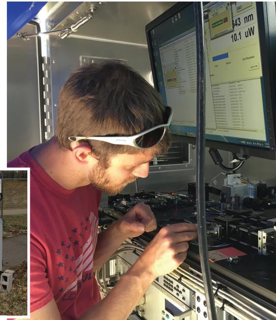
A differential-absorption lidar (DIAL) system (inset) has been developed by NASA using Photodigm distributed Bragg reflection (DBR) injection-seed lasers. (Image credit: NCAR)
