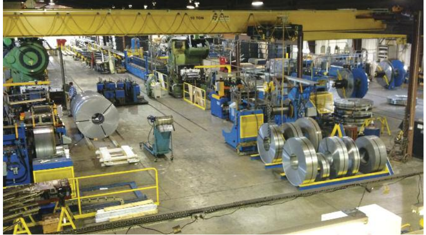
These slit coils are being used on some of Hynes’ 38 roll forming lines.
