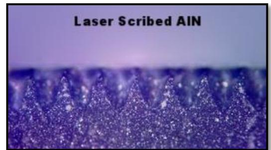
If a smoother edge is required, consider a diamond sawn edge or laser cut and subsequently annealed or clean fired edge for higher edge quality.
