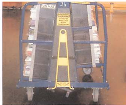
The newer spring-loaded tow bar was designed to eliminate bending and lifting the detachable tow bar.
