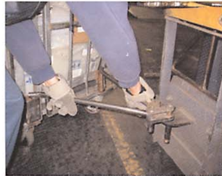
The newer spring-loaded tow bar was designed to eliminate bending and lifting the detachable tow bar.
