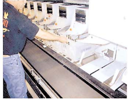
The AFSM 100 is designed to enable you to slide the full trays.
