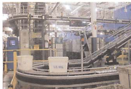
The Tray Management System eliminates much manual lifting. Among other features, trays are delivered at waist height (above right).
