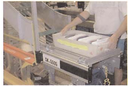
The Tray Management System eliminates much manual lifting. Among other features, trays are delivered at waist height (above right).
