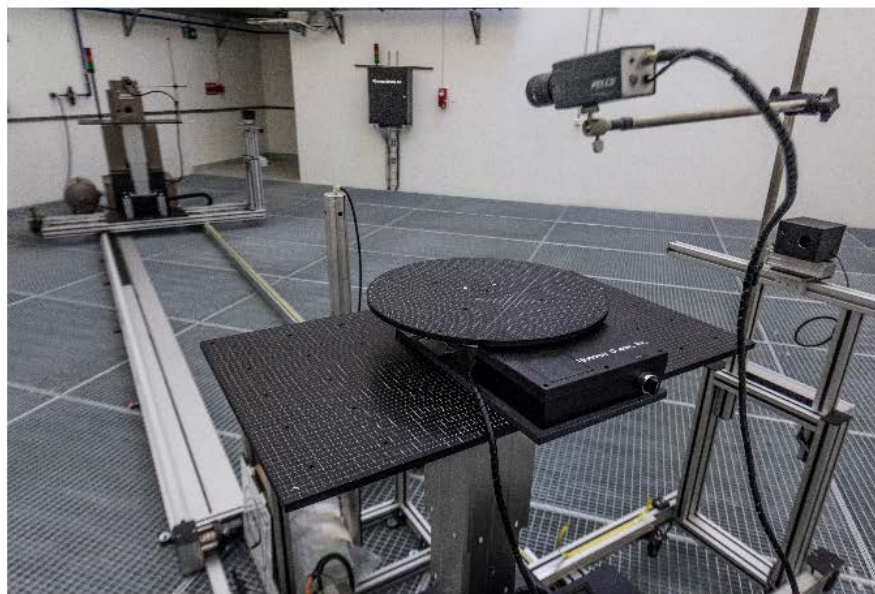
New four-axis calibration bench for radiation protection instruments.
