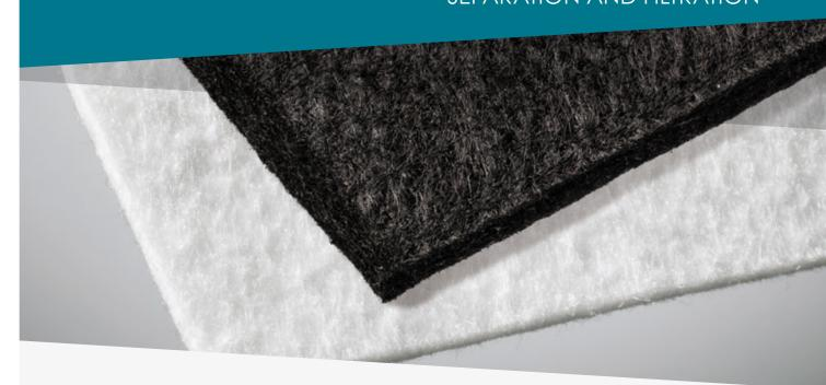
Enka-Tex N nonwovens are a range of needle-punched and thermally bonded geotextiles that offer the highest levels of engineering performance and quality standards. It incorporates products with superior puncture resistance compared with other needle punched nonwoven products of comparable weight. The range is used in various applications including site access roads, hard standings, road and railways, drainage blankets, car parks, landfills and coastal engineering.
