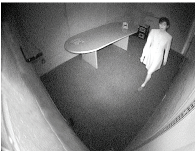
The EX36N uses active-infrared to ‘invisibly’ illuminate a room, important for sleep research.
