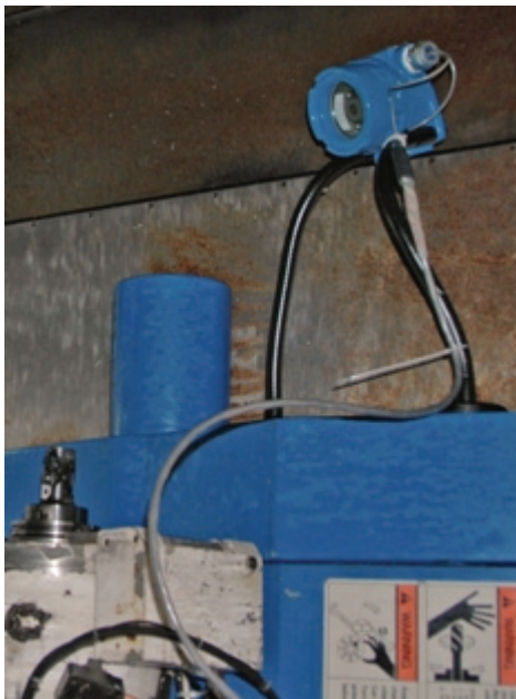
Cameras installed for monitoring help Boeing Research and Technology improve machining control programs.
