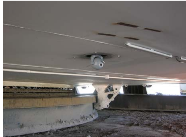
MIC1 provides surveillance for critical blind spots for Dragline operators.
