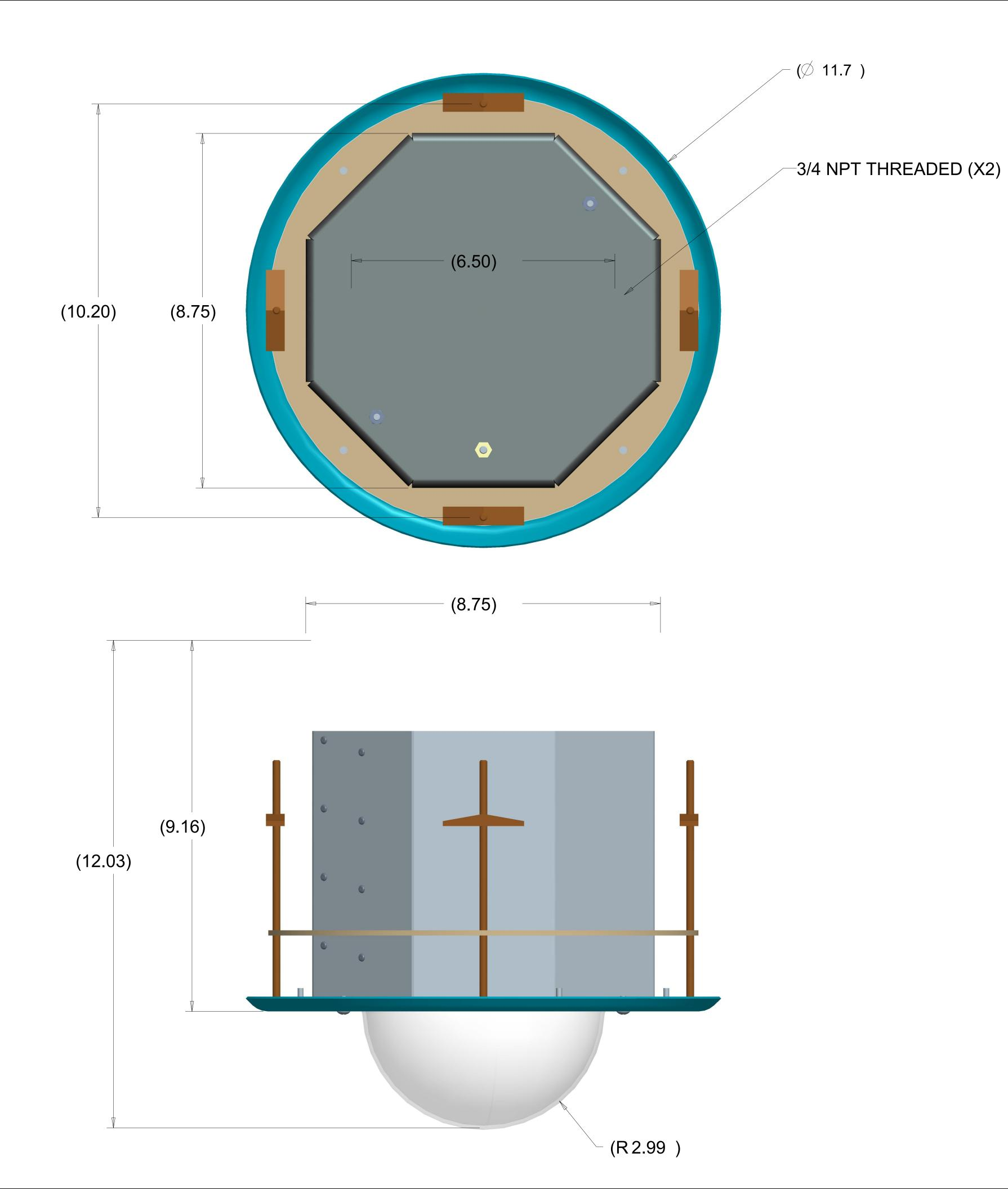
RECESSED OCTAGON CAN ALUMINUM WELDMENT POWDER COAT PAINT
