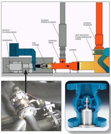
INSTALLATION: The DFT 3" ASME 600# 316SS/316SS GLC with sizing, soft seat, and special spring on the water injection line near the turbine in the box (approximate location indicated by arrow in above picture).
