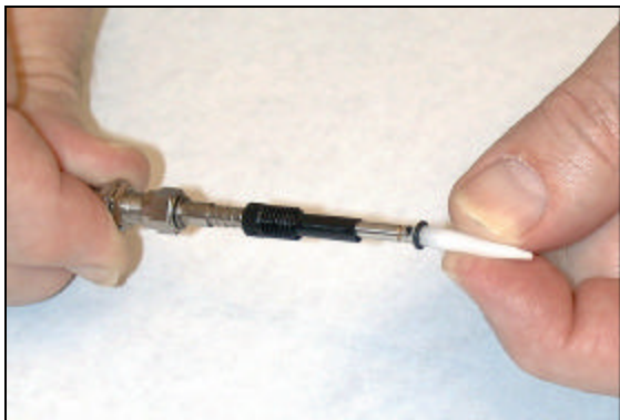
Installing the o-ring on the 125/FO probe.
