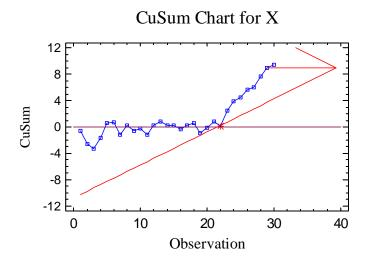
Assuming that a process is designed to operate at a mean level  $\mu$ , the *CuSum V-Mask* procedure plots the cumulative sum of deviations from the mean. For individuals data, the cusum is defined
