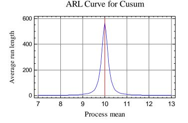
The ARL curve plots the average run length (average number of values plotted up to and including the first point beyond the control limits) as a function of the true process mean. Assuming that the process mean suddenly shifts to a new value, the plot shows how long it takes on average until an out-of-control signal is generated. For very small shifts, it can take in excess of 400 points on average to detect the shift. At a shift to  $\mu = 11$ , the ARL is approximately 10.5.
