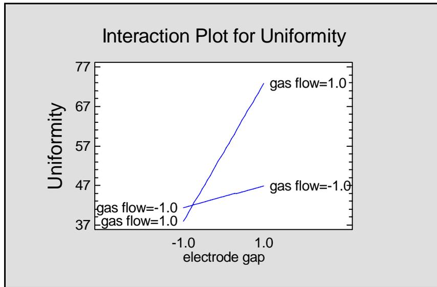
Figure 27: Interaction Plot for Electrode Gap and Gas Flow
