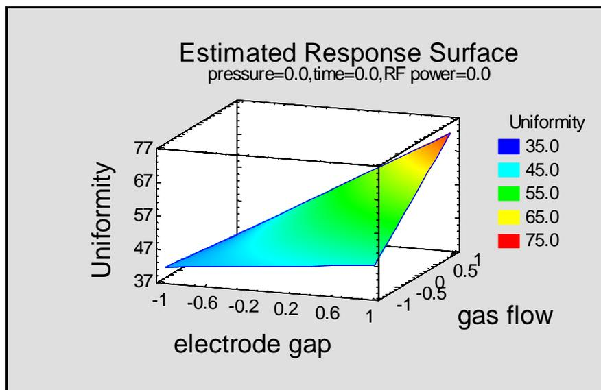
Figure 28: Uniformity versus Electrode Gap and Gas Flow
