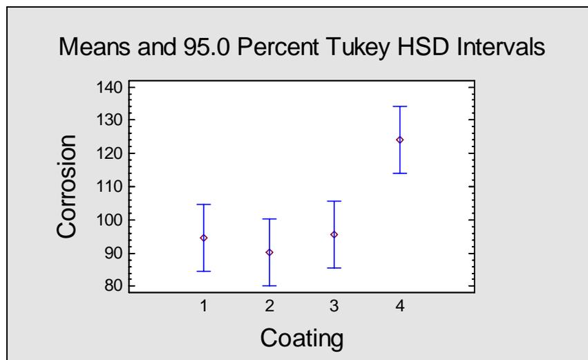
Figure 12: Means Plot for Coating
