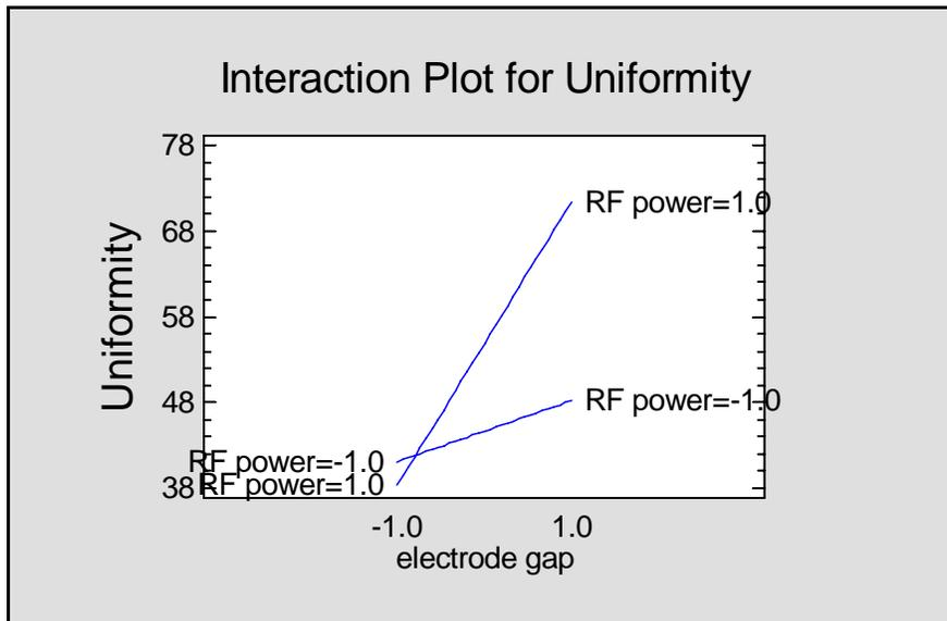
Figure 31: Interaction Plot for Electrode Gap and RF Power
