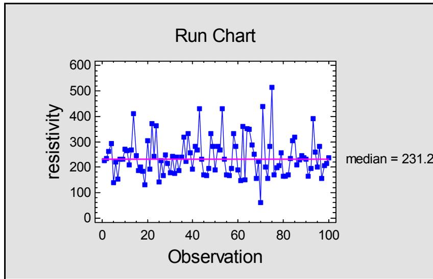
Figure 3: Run Chart for Resistivity Measurements
