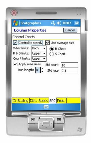
The *Count limits* pulldown list indicates whether lower and/or upper control limits should be plotted for the charts. The *Use average size* field indicates whether the average sample size should be used to generate horizontal control limits, or whether individual sample sizes should be used (resulting in jagged control limits if the sample sizes are not all equal).
