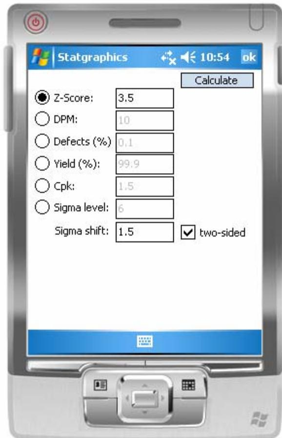
To use the calculator, select one of the six radio buttons, enter a value in the corresponding edit field, and press the *Calculate* button. The corresponding values of the other quality performance metrics will be displayed to the right of the edit fields.
