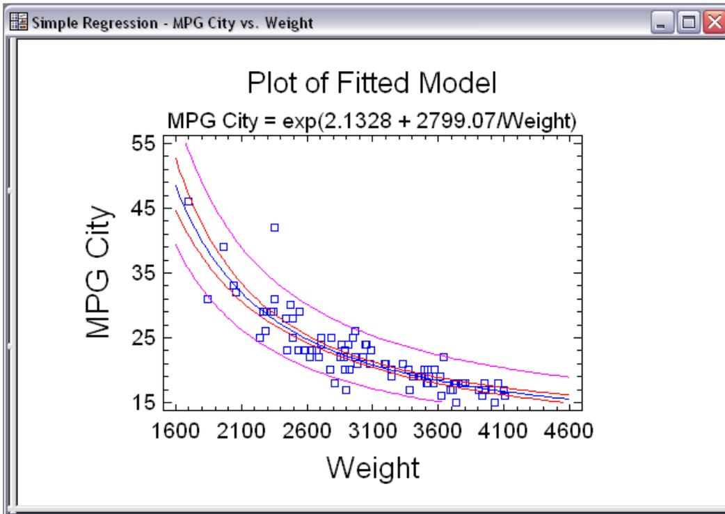
Figure 3-7. Fitted S-Curve Model
