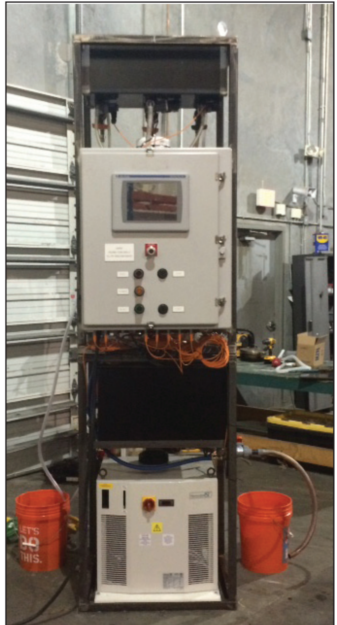
Pfannenber CC 6301 chiller in a rack-mount Ferrator prototype.
