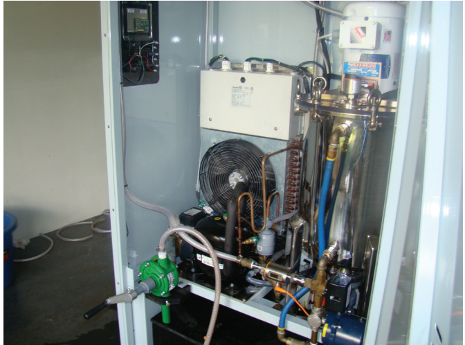
Pfannenberg open-frame chiller inside packaged Ferrator.
