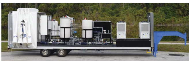
Pfannenber chillers on trailer-mounted Ferrator.
