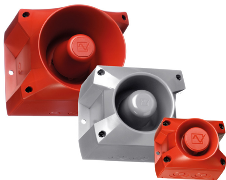
PATROL sounders offer a selection of 80 different tones, permitting the user to select a unique, identifiable signal for a specific alarm event. Additionally, with four stages of alarm, one unit can output up to four different tones to signify different events.
