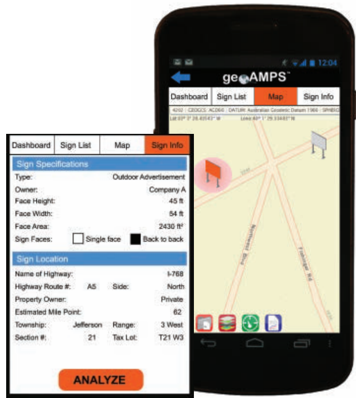
Figure 3: With web-based software, DOT staff can use mobile devices for on-site analysis of permit applications and receive feedback in real time.
