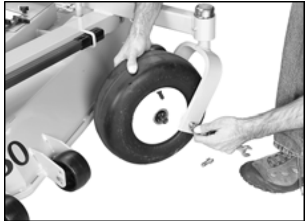
Deck Caster Wheel Installation
