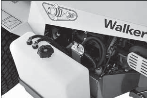
Fuel Selector Valve - Model MBS26
