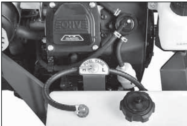
Fuel Selector Valve - Model MBS
