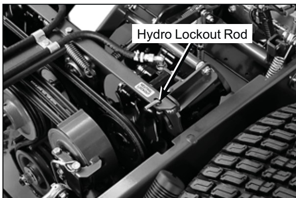
Hydro Lockout Rod - Normal Operating Position
