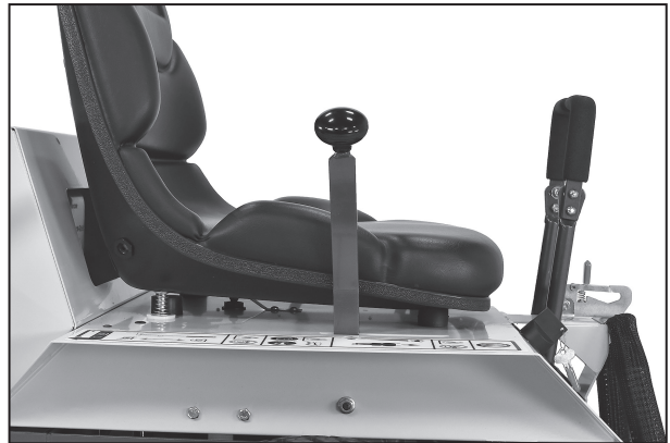
Correct FSC Lever NEUTRAL-PARK Position
