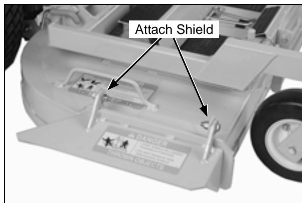
Deck Discharge Shield Installation
