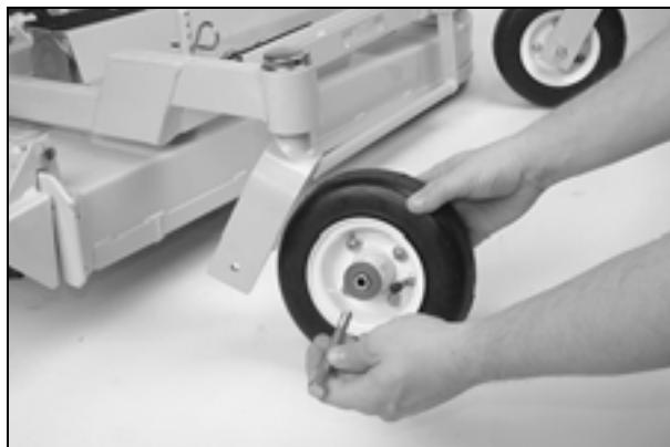
Deck Caster Wheel Installation
