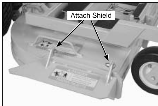
Deck Discharge Shield Installation
