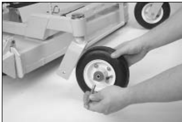
Deck Caster Wheel Installation
