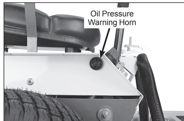
Warning Horn Location
