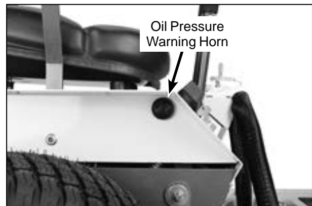
Warning Horn Location
